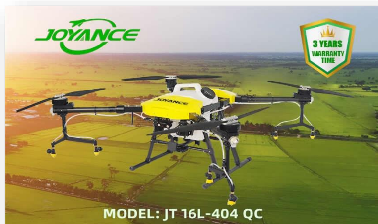
Figure 2. The Joyance 16 liter drone used with dual conventional nozzles
