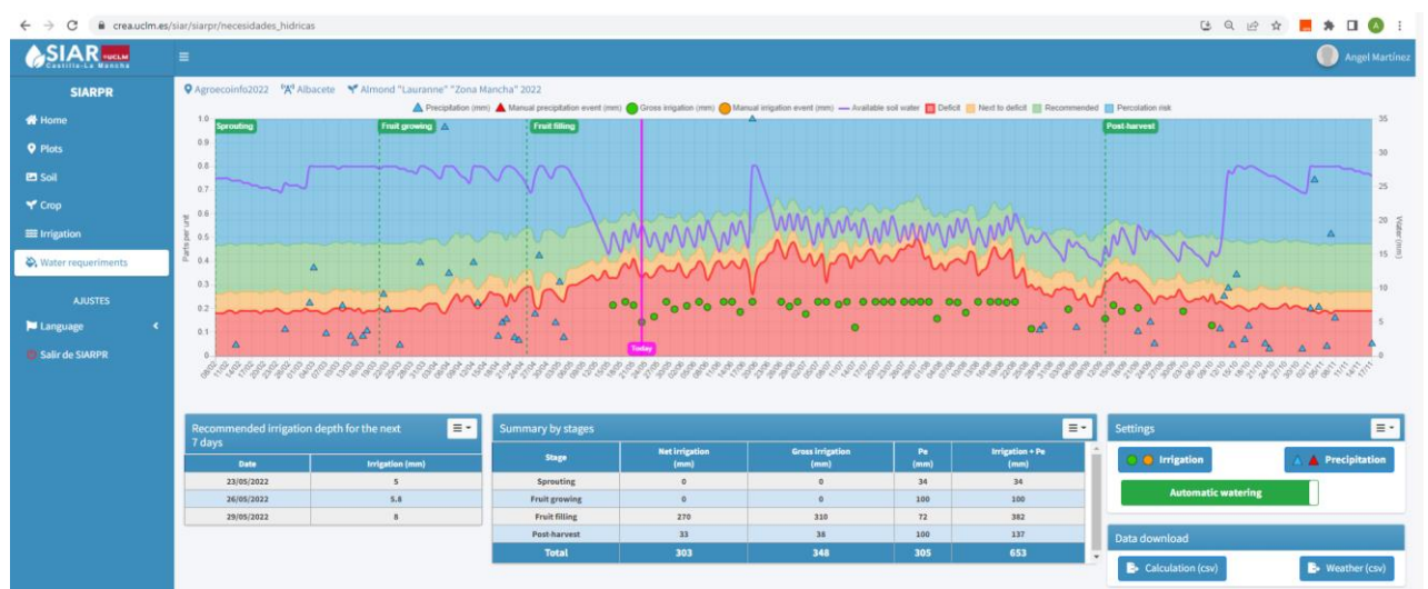
Figure 5: Evolution of available water simulated by “MOPECO irrigation scheduling” tool in 2022 for almond (20% deficit) (Main Y axis: Deficit: 1-p, where p is the fraction of TAW (Total Available Water) that a crop can extract without suffering water stress; Available water. Secondary Y axis: Gross irrigation; Precipitation.
