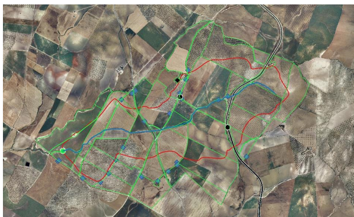
Figure 1 Orthophoto of year 2016 showing the catchment boundaries (red), main channel (blue), farms boundaries (green), location of the hydrological station (green circle), hydrants (blue squares) and the rain gauges (black circles) in the Catch-Lab.
