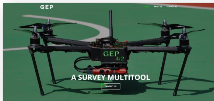
Figure 3. The surveillance drone used to establish NDVI maps
