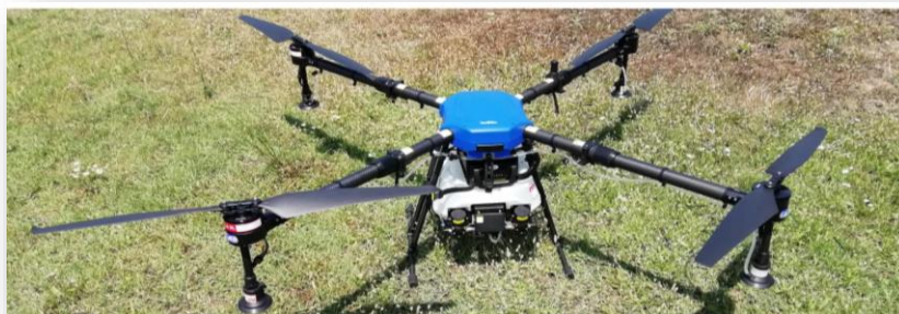
Figure 1. The Topxgun 16 liters drone used for spraying, with centrifugal nozzles.
